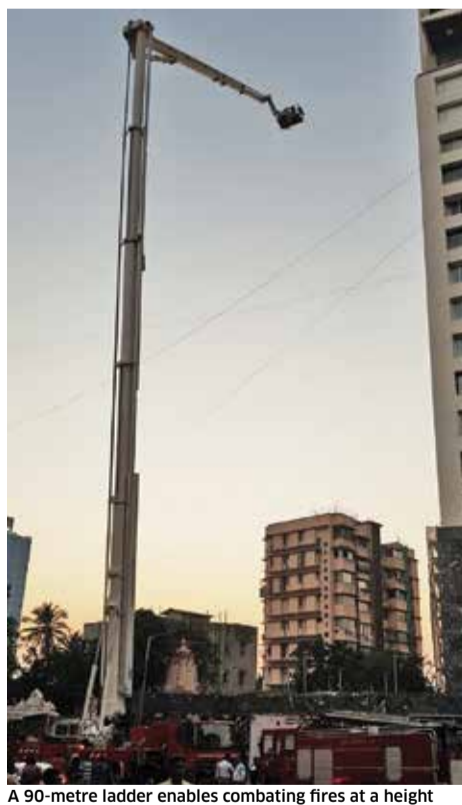
A 90-metre ladder enables combating fires at a height
