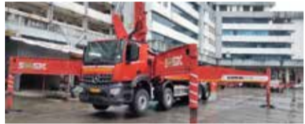
Newly included 55 meters Flexible Water Tower Vehicle for effective fire-fighting in inaccessible areas
